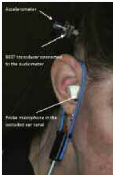
Figure 1. Setup for the two "real-ear-like" approaches to verifying Baha
